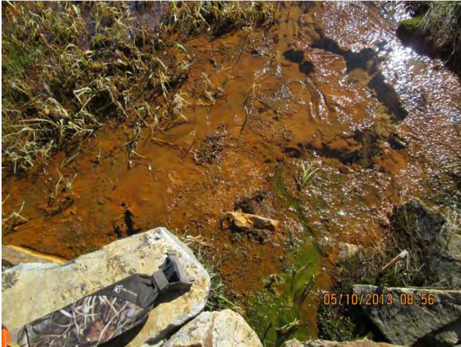
Figure 4I. Photo of the North Keyway Dam seep (YP-S-8) from the Surface Water Quality Baseline Study, Appendix G, May 2013 Site Photos, page 16. Photo caption reads, "YP-S-8, North Keyway Dam seep. Close-up looking east and downstream at seep source emerging from base of dam. May 2013."
